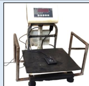
Device based on IOT System for Authenticating Milk Yield Recording of Dairy Animals
